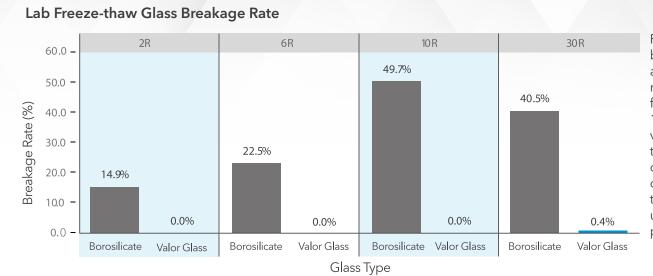
Freeze-thaw glass breakage rates using aggressive 15% mannitol with 50% fill volumes of 2R, 6R, 10R, 30R borosilicate vials compared to matching Valor containers. Study was conducted at -100°C to room temperature utilizing 1,000 vials/ pedigree.
